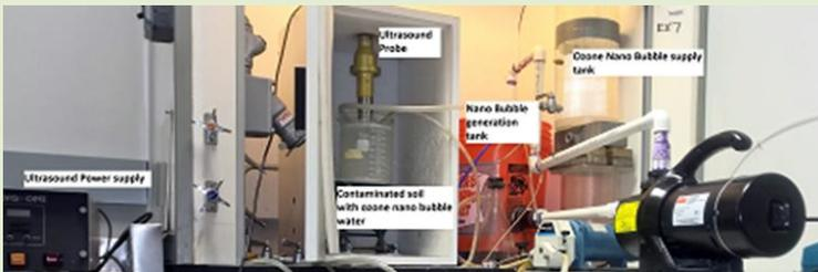
In order to validate and to optimize the proposed technology bench scale tests will be performed followed by statistical analysis. The key factors that contribute to the removal efficiency will be identified in bench scale tests and full factorial design will be performed to generate removal efficiency data for statistical analysis. In addition, stability of nano bubbles will be investigated to
