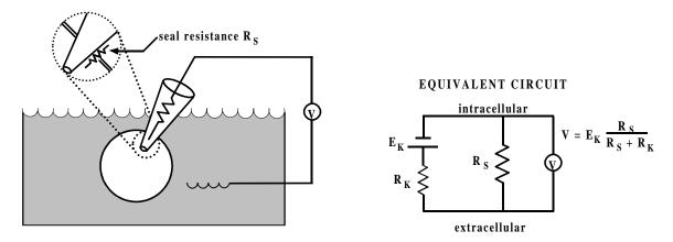
Figure 1-16. Intracellular Electrode Measurement
