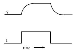
Figure 1-14. RC Parallel Circuit Response
