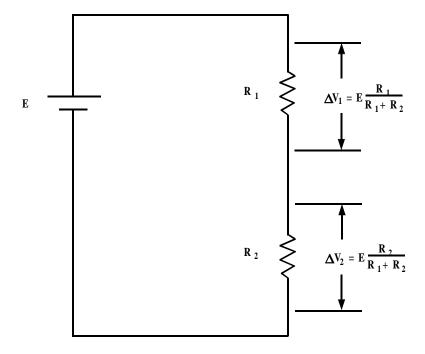
Figure 1-7. A Voltage Divider
