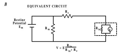
**Figure 1-8.** Representative Voltmeter with Infinite Resistance Instruments used to measure potentials must have a very high input resistance R<sub>in</sub>.
