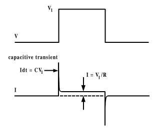
**Figure 1-15.** Typical Voltage-Clamp Experiment A voltage-clamp experiment on the circuit of Figure 1-13.
