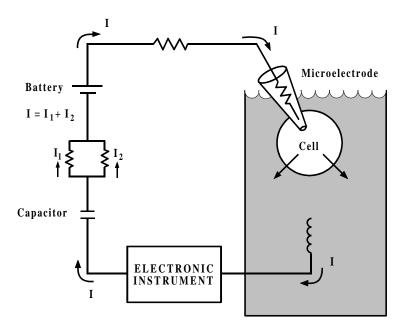
Figure 1-2. A Typical Electrical Circuit
