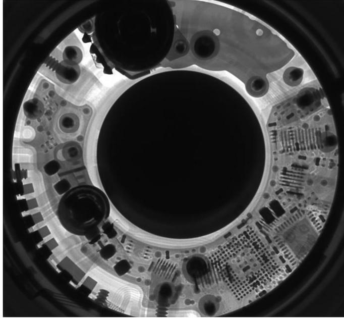
*Photo: A Canon DSLR Lens (24mm f2.8 pancake lens) is imaged at resolution of ~20 micron using a Bruker SkyScan microCT scanner. The camera's outside ring is composed of thin metal, while the darker inner circle of the camera lens is composed of dense glass. Credit — Mathew Schwartz/NJIT*
