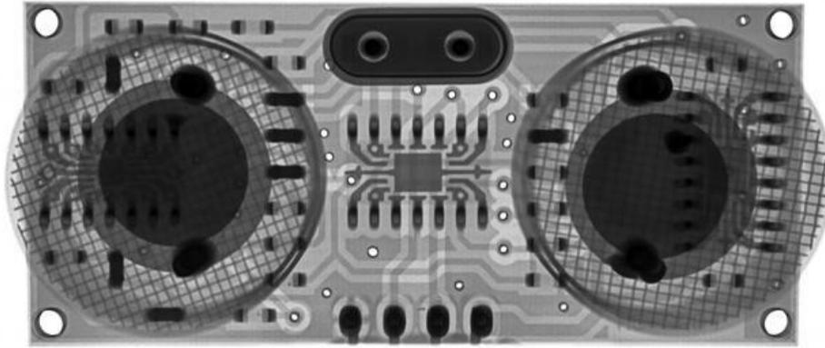
*Photo: A black and white microCT scan image of an ultrasonic sensor at resolution of ~15 micron. Credit — Mathew Schwartz/NJIT*
